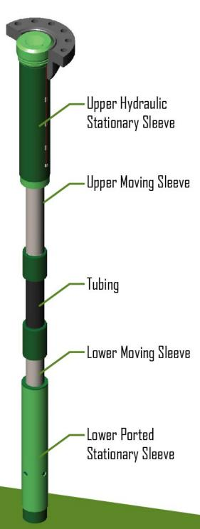
Slip String Flush Tool: NO FLUSHBY TRUCK NEEDED!
